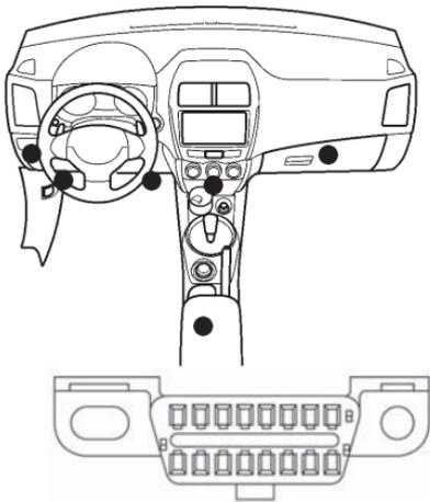
When connecting the diagnostic connector with the engine running, on some 1996-2008 production year cars ABS, ESP, etc. indicator lamps may start flashing. Blinking of indicator lamps means that these systems are disabled and do not work! Be careful! In this case, we recommend connecting the diagnostic scanner only with the ignition off.
